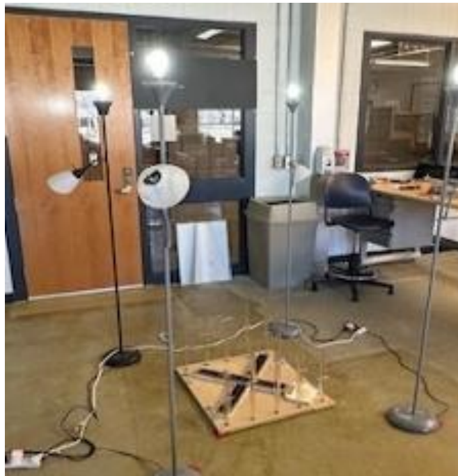
Figure 5. The figure shows the placement of the measuring panel while it was being calibrated. The four LED lights were used to provide near uniform intensity on the panel.
