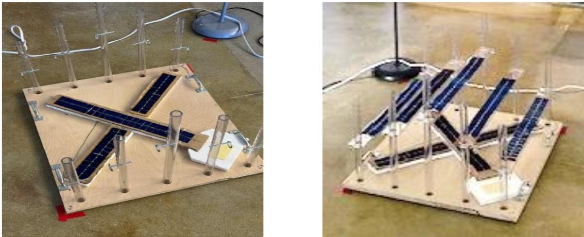
**Figure 4.** Solar cage and measuring pane structure. (a) The figure shows only the measuring panel on the base; (b) The solar cage is placed on the floor; the measuring panel lies on the base of the cage.
