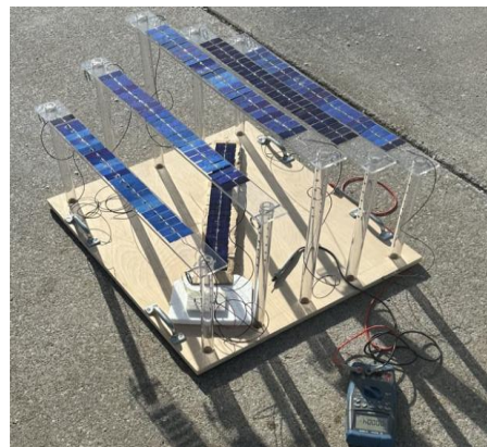
Figure 2. 5-panel structure with adjustable height. The measuring panel sits on the ground for experiments. The 5 panels are placed at the top level in the figure.
